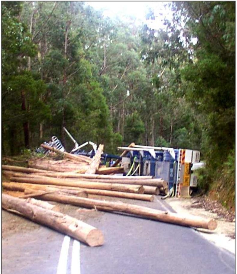
*A log truck has a high centre of gravity and therefore it does not take much to make it roll. Photo courtesy VicRoads.*
